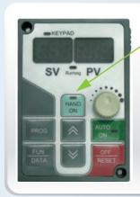
If Pump A is in automatic constant pressure mode, in case of emergency, the pump must be separated from automatic constant pressure mode the user can directly press the "HAND ON" button to manually reduce the frequency from the operation frequency memorized in automatic constant pressure mode to stop system.
